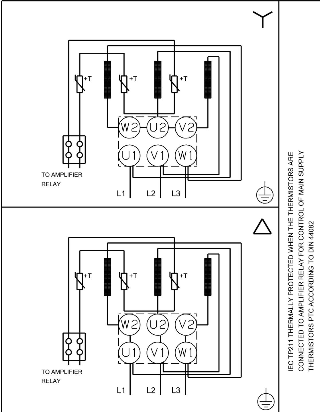
IEC TP211 THERMALLY PROTECTED WHEN THE THERMISTORS ARE
